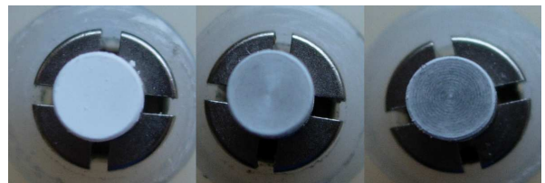
Figure 14: The SEM targets after the second flow test, third is left-most, first right-most. The second showing a lighter coating of salt than the third, and the first only a slight dusting.
