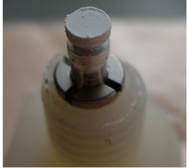
Figure 12: The third SEM target after the test, showing a thick coating of salt.
