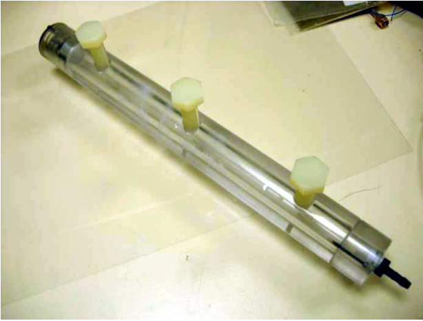
Figure 3: The electrostatic precipitator was machined from perspex, with a piston at the inlet to prevent contamination.
